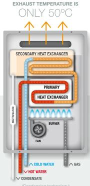
(Condensing technology) Thermal efficiency = 90~96%
